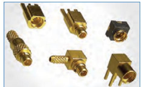
**MMCX** MMCX (also called MicroMate™) is a micro-miniature connector series with a snap-lock mechanism allowing for 360-degree rotation. MMCX connectors conform to the European CECC 22000 specification. The MicroMate family of products is a 6 GHz 50  $\Omega$  interconnect. A range of connectors are available, including surface mount, edge card, and cable connectors. Common applications include broadband, instrumentation, and telecommunications.
