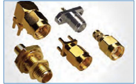
**SMA** SMA is an acronym for sub-miniature version A and was developed in the 1960s. It uses a threaded interface. 50 Ω SMA connectors are semi-precision, subminiature units that provide excellent electrical performance from DC to 18 GHz. These high-performance connectors are compact in size and mechanically have outstanding durability. SMA connectors are used in phase array radar, test equipment, ILS landing systems, and other instrumentation.
