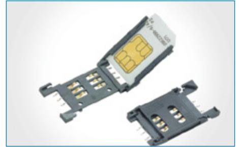
**SIMLOCK®** Amphenol's SIMLOCK® was designed for SIM/SAM card applications. The SIMLOCK features dimensions only slightly larger than the SIM card. The closed system with integrated card guidance critical card tolerances as per GSM 11.11. The polarization notch does not allow incorrect card positioning. Suitable for automatic assembly processes: pick & place, tape & reel packaging, and SMT solderable.
