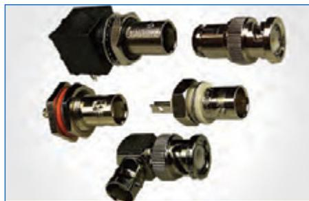
**BNC** Developed in the late 1940s as a miniature version of the Type C connector, BNC stands for Bayonet Neill Concelman and is named after Amphenol engineer Carl Concelman. The BNC product line is a miniature quick-connect RF connector. It features two bayonet lugs on the female connector. BNCs are ideally suited for termination on miniature and subminiature coaxial cable, including RG-58, 59, RG-179, and RG-316.
