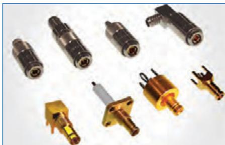
**1.0/2.3** The compact design of the 1.0/2.3 series permits dense connector packing. They are ideally suited to applications where space saving is critical. Versions are available with threaded coupling mechanisms, which provide positive mating, or a unique push-pull coupling system, which allows quick installation. Amphenol 1.0/2.3 coaxial connectors are 50  $\Omega$  units operating from DC-10 GHz. Common applications are amplifiers, base stations, routers, and switching equipment.
