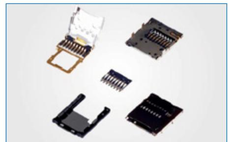
**Micro-SD Connector** Amphenol produces a wide variety of micro-SD and mini-SD memory card connectors. These connectors are available in hinged and non-hinged varieties as well as in a push-push version. They are typically used in a wide range of portable electronic devices including mobile phones, smart phones, PDAs, MP3 players, GPS devices and video game systems.
