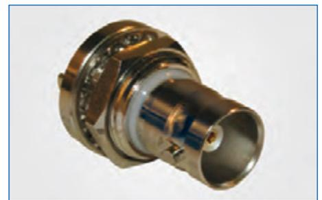
**Mini-BNC** The Mini-BNC is designed for wireless applications for higher connector densities while preserving the positive characteristics of the Amphenol full-size BNC's for 75 Ω systems., allowing 40% more interconnects in the same area. The Mini-BNC connector interface offers a 75 Ω impedance with acceptable return loss up through 1 GHz and a positive bayonet locking coupling mechanism.
