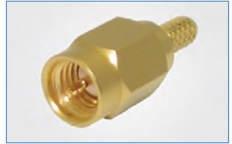
**SSMA** The SSMA connector is designed to be a space-saving alternative to the standard SMA originally designed for use with .085 semi-rigid cable. The male contact was designed to be the same size as the cable conductor so that it could be used as the mating pin for optimized VSWR. This interface is available with 50 Ohm options and gold plating is standard.
