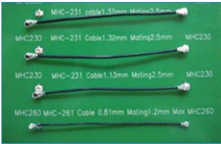
**AMC Connectors, Jumpers and Adapters** Amphenol Micro Coaxial (AMC) connectors, jumpers and adapters are ultra-low profile (2.5mm mating height) RF connectors with a small footprint (3mm x 3mm). The AMC series offers easy snap-on/off mating, 50Ω impedance, and DC - 6 GHz frequency range. The series is also 100% compatible with the U.FL interface.
