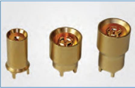
**AFI** The AFI connector interface is a solution for board-to-board RF applications. It utilizes a proprietary configuration that allows for industry leading "float" to compensate for the axial and radial misalignment due to packaging tolerances. This industry-leading float results in a maximum misalignment allowed by the system of .030" (0,8 mm) radial and .040" (1,0 mm) axial.
