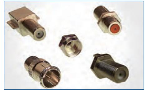
**Type F** Amphenol knows that low-performance F receptacles could not be used in high-speed cable modems and customer interface units (CIUs). The industry has challenged connector manufacturers to develop high-performance connectors featuring -30 dB return loss at 1 GHz – Amphenol has met this challenge. Our high-performance F-connectors comply with a 3/8-32 thread specification. Primary applications are for cable television (CATV), set-top boxes, and cable modems.
