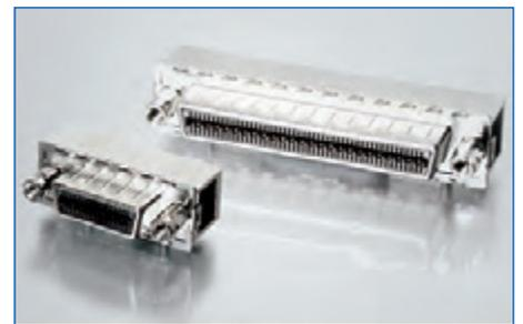
**Infinity Connectors** The Infinity series of receptacles is compliant with SFF-8470 specifications, and is available in both 4x and 12x configurations. Lanyard latching mating styles are available for use with CX4 and InfiniBand applications, as well as Screwlock mating styles for use with SAS, Fibre Channel and 10Gb Ethernet applications.
