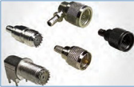
**Mini-UHF** Mini-UHF is a miniature version of the UHF connectors that were developed for use in the radio industry. Mini-UHF connectors are used as coaxial interconnects in cell phones, automotive systems, and similar applications where size, weight, and cost are critical. Mini-UHF connectors terminate to RG-58, RG-58A, RG-58B, RG-58C, and Belden 9258 cables. Crimp-type cable plugs and jacks are available, as well as panel and PCB receptacles.
