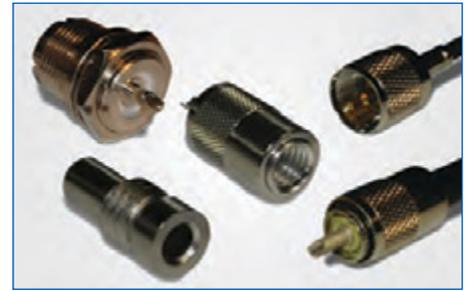
**UHF** Invented for use in the radio industry in the 1930's, UHF stands for Ultra High Frequency. While at the time 300 MHz was considered high frequency, these are now general purpose connectors for low frequency systems from 0.6 - 300 MHz. UHF connectors feature optional reducing adapters which accommodate a wide range of popular coaxial cables.
