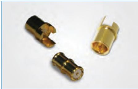
**SMP** Amphenol offers a solution for high frequency, high data rate applications in the SMP line of RF connectors. The SMP connector features a subminiature with a frequency range of DC to 40 GHz. It is commonly used in miniaturized high frequency coaxial modules and is offered in both push-on and snap-on mating styles for quick installation.
