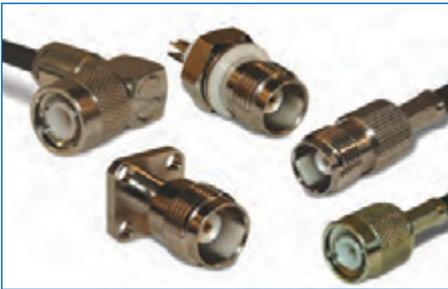
**TNC** The TNC connector series features a miniature, threaded weatherproof interface with a constant 50  $\Omega$  impedance and operates from 0 - 11 GHz. The TNC is available in standard and reverse polarity configurations. Reverse polarity is a keying system accomplished with a reverse interface, and ensures that reverse polarity interface connectors do not mate with standard interface connectors.
