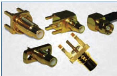
**SMC** The SMC connector features a medium-sized 50 Ω threaded interface designed to meet of MIL-STD-348 standards as generated by the US Air Force. It utilizes die cast components on non-critical areas to provide a low cost solution. The series offers a 10-32 screw-on (threaded) coupling mechanism, allowing performance to 10GHz with low reflection.
