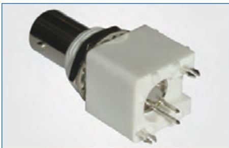
**Valox** Amphenol RF BNC Valox Connectors are isolated from the panel via a Valox housing to provide high performance in RF and microwave communications. BNC Valox Connectors feature a proven, easy-to-use interlocking interface that integrates seamlessly into any 50-ohm or 75-ohm RF system. These connectors are well-suited for instrumentation, broadcasting, and network applications.
