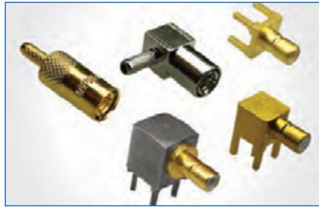
**SMB** Amphenol's SMB connectors conform to the requirements of Mil-C-39012, and the interface is in compliance with MIL-STD-348. Available in 50Ω and 75Ω, the SMB provides broadband capability through 10 GHz with a snap-on connector design and utilizes die cast components in non-critical areas to provide a low-cost solution.
