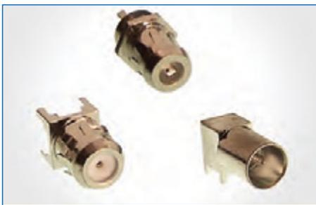
**Type G** Our Type G connector is a slide-on alternative to the Type F with 15A continuous current rating. The Type G complies with the MIL-STD 202 specification for vibration, shock, thermal shock, moisture resistance, and salt spray. The Type G has an impedance of 75 Ω — ideal for CATV applications. The Type G line consists of Bulkhead Mount Jack Receptacles and PCB Mount Jack Receptacles.
