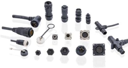
The Ceres Series waterproof connectors are available as a receptacle, receptacle connector with cable, and over-molded with cable. The field installable options are available in multiple sizes mini, standard, middle, and large. The Ceres waterproof connectors offer  $\leq 10\text{m}\Omega$  contact resistance,  $\leq 100\text{M}\Omega$  at DC500V insulation resistance, and at least 2000 mating cycles.
