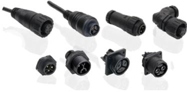
Power Connector Series offer up to 50A current rating and feature a robust, high-density crown spring terminal design. Hybrid-type Power Connectors offer 2A signal current in addition to up to 50A power and provide a three-points lock bayonet mating style. The Power series is UV resistant and UL 94V-0 rated. The series also provides IP67 ingress protection when mated and is ideal for use in electric bikes, lighting systems, industrial automation, and broadband wireless access.
