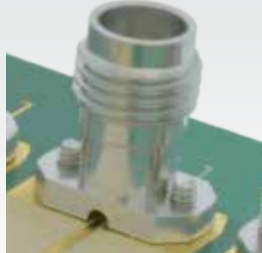
Launches directly to a Coplanar Waveguide or Microstrip trace, which exits through a small mouse hole on the side
